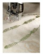
stitch, then while the machine is still running, press against the knee lifter to widen your stitch to a 9mm zigzag. Release pressure to gradually return to a straight stitch for a tapered finish. This advanced feature opens up amazing new possibilities for creation expression with free motion quilting, thread painting, raw edge appliqué, free motion monogramming, and more.
