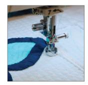
the Ruler Work foot (QR) to safely follow along the guiding edge of precision cut templates.
