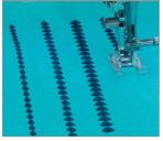
with 9mm stitch width, this sort of bold detail can be easily appreciated.
